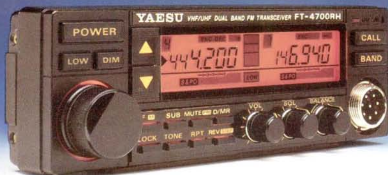
FT-4700RH control head (1 5 / 16 " x 5 7 / 8 " x 1")
